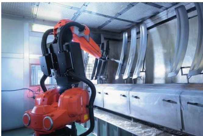
▲ Figure 6.18 Robot with spray gun end-effector
